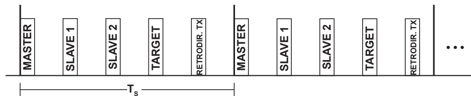
Figure 2.16: A timeslot diagram showing the periodic exchange of messages in the experimental setup.
