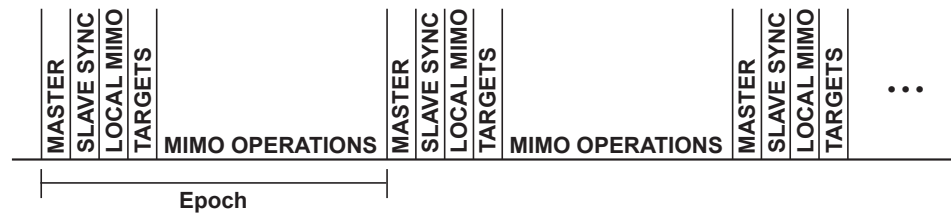
Figure 4.2: A timeslot diagram describing the activity that must occur during each epoch.
